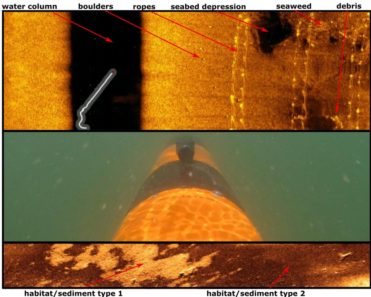
Figure 1 (Top) Acoustic side-scan sonar image indicating boulders, seaweed and debris on the seabed and seaweed ropes in the water column via high acoustic amplitudes (bright colors). Dark colors indicate areas with no or very little acoustic energy returning to the sonar as for the water column below the sonar and a depression on the seabed. (Middle) AUV travelling through the murky water. (Bottom) Acoustic image showing a heterogeneous seabed with two different habitat/sediment regions.
