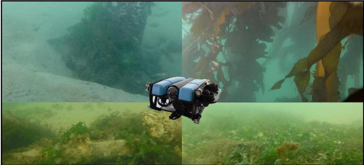
Figure 2 ROV camera footages. (Top left) Scouring around farm foundations, (top right) growing seaweed, (bottom left) lost seaweed and debris on the seabed and (bottom right) extensive field of seaweed.
